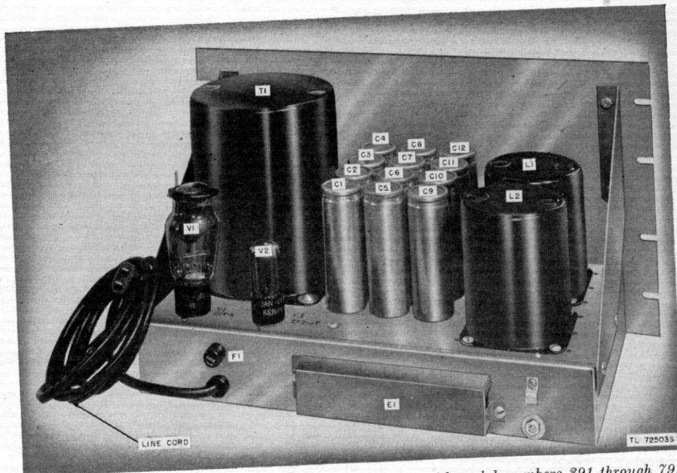
Figure 43.2 (Added.) Power Supply Unit RA-74-D, with serial numbers 391 through 791, Order No. 6036-Phila-48, chassis, top view.
